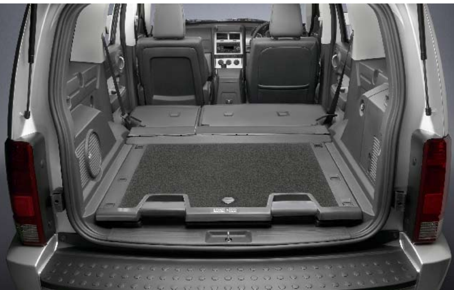
LEFT: A great gimmick is the practical sliding panel in the rear, dubbed Load 'n Go.
